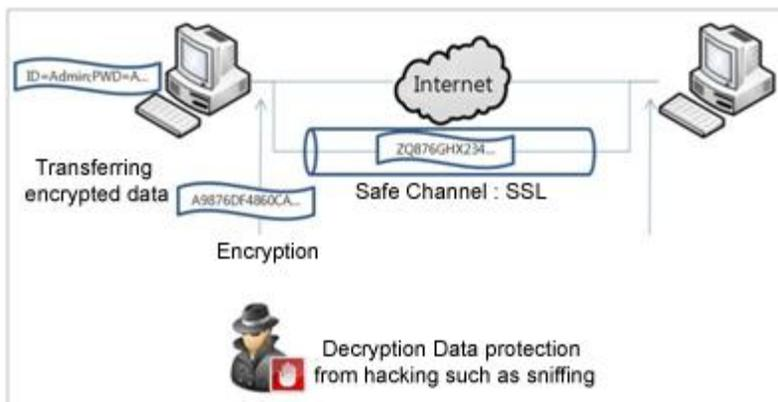
The below data should be protected while supporting the remote computer: Screen Sharing, Keyboard/Mouse control, Text Chat, File Transfer, data created by remote support functions.
